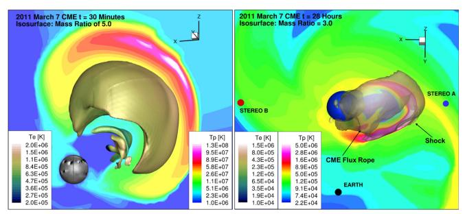
Figure 12. Left panel: CME-driven shock structure in SC at t = 30 Minutes. Right panel: CME-driven shock structure in IH at t = 28 hr. The isosurface in SC shows the density ratio of 5. The isosurface in IH shows the density ratio of 3. The background shows the proton temperature, and the color scale on the isosurface shows the electron temperature. The Earth, STEREO A, and STEREO B positions are shown in IH with different color spots.
