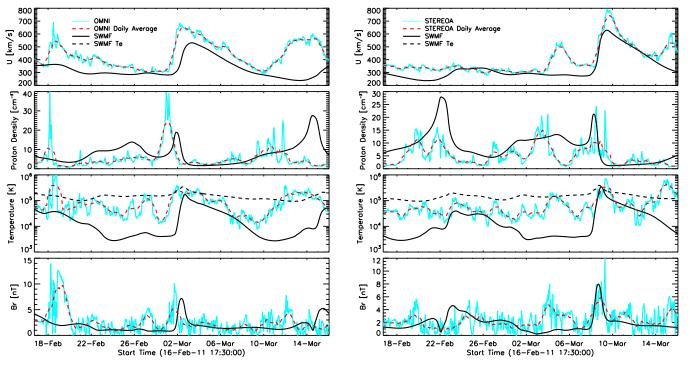
**Figure 2.** Comparison of OMNI and *STEREO A* observed solar wind speed, proton density, proton/electron temperatures, and magnetic field with the steady state model output for CR2107.
