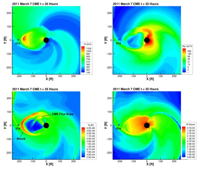
Figure 13. Radial velocity, proton density, proton temperature, and total magnetic field of the simulated CME at t = 35 hr.
