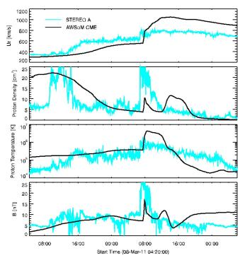
**Figure 14.** Comparison of the CME in situ observation with the simulation for radial velocity, proton density, proton temperature, and total magnetic field.
