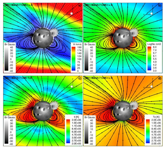
Figure 4. Meridional slice of the SC showing the (a) radial velocity, (b) plasma density, (c) proton temperature, and (d) electron temperature at t = 0 after GL flux rope implement. The radial magnetic field is shown at  $r = 1.03 R_{\odot}$  with gray scale. The white boxes in the velocity map show the grid information for the steady state simulation. The black lines show the projected magnetic field lines on the meridional slice.
