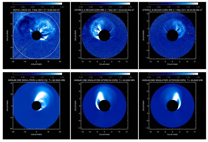
Figure 9. Comparison between the LASCO C3, COR2A, and COR2B white light images, with the model synthesized images for the 2011 March 7 CME event. The color scale shows the white light total brightness divided by that of the pre-event background solar wind.
