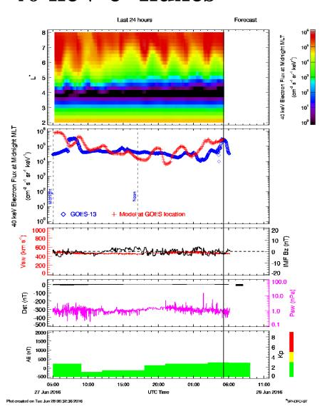
**IMPTAM**: traces **electrons** (< **200 keV**) with arbitrary pitch angles (**drift approximation**) from the plasma sheet to the inner L-shells in time-dependent magnetic and electric fields
