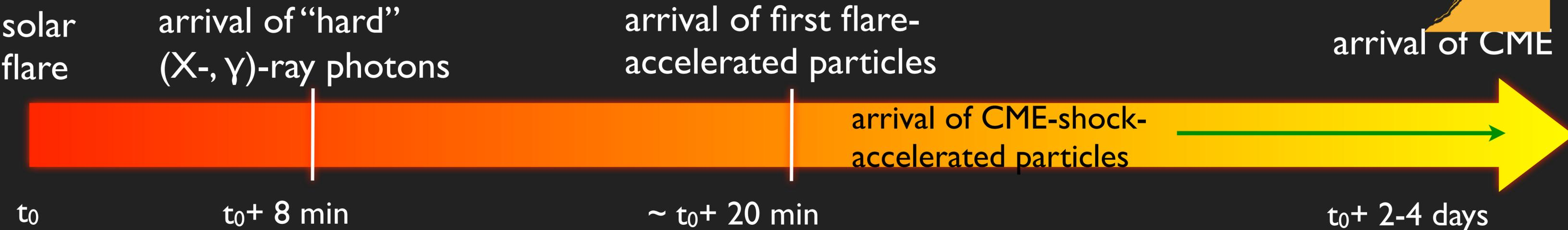
Hard flare photons and non-thermal particulate (mostly protons  $> 10 \text{ MeV}$ ) affect humans beyond LEO and on solar system bodies lacking an atmosphere. Damages in space-based electronics, radio blackouts, etc., can occur as a result of flares
