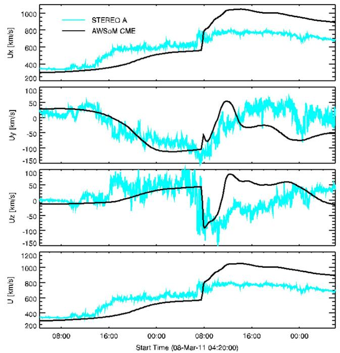
**Figure 17.** Comparison of the CME in situ observation with the simulation for  $V_x$ ,  $V_y$ ,  $V_z$ , and total velocity field.
