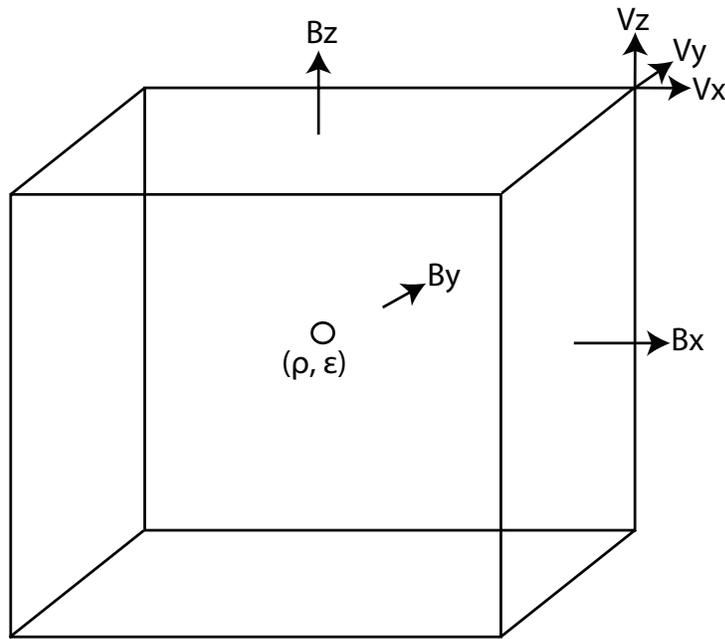
Figure 3: Staggered grid locations for SWIFT variables.
